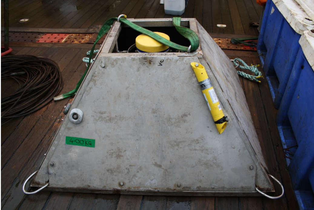
Figure 3.5: Example ADCP seabed frame
