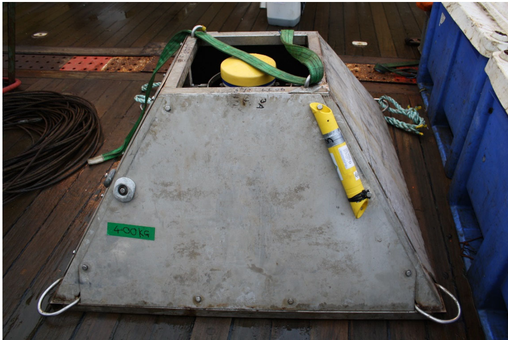
Figure 3.5, Figure 3.6 and Figure 3.7). The dimensions of the ADCP devices and the anchor blocks to be placed on the seabed are 1 m 2 .
